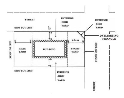
DISTANCE AB REPRESENTS THE DEPTH OF THE REQUIRED YARD MEASURED AS LEAST HORIZONTAL DIMENSION BETWEEN LOT LINE AND NEAREST PART OF MAIN BUILDING. DISTANCE AB MUST BE THE MINIMUM DISTANCE SPECIFIED DISTANCE.
